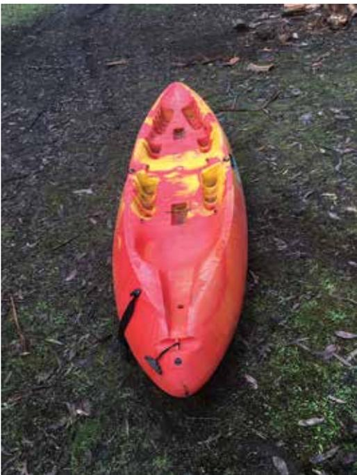
**Figure 3 - Sit on top kayak supplied to Brauer College. Note capacity for two persons. Sit on top style of kayak is of a sealed hull configuration that provides integral buoyancy without the need for additional buoyancy.**
