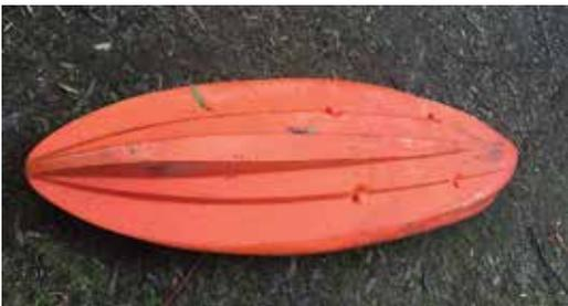
**Figure 2 - Bottom of kayak, keel provides increased directional stability and helps reduce leeway (drift under the influence of wind)**
